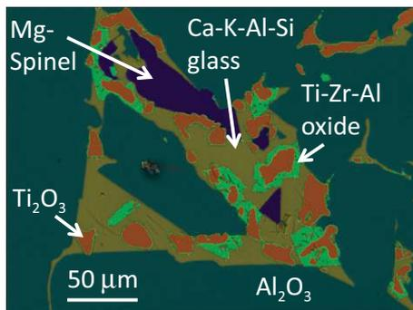
**Figure 2.** Energy-dispersive X-ray spectroscopy–scanning electron microscopy composite element map of type S melt pocket in corundum matrix from Mount Carmel, Israel, showing tistarite ( $\text{Ti}_2\text{O}_3$ ), some rimmed by Ti-Zr-Al oxide, and crystal of Mg-spinel in matrix of Ca-Al-Si glass (Table 1). Note combination of straight and lobate boundaries to melt pocket, defined by crystal faces of adjacent corundum ( $\text{Al}_2\text{O}_3$ ) crystals.
