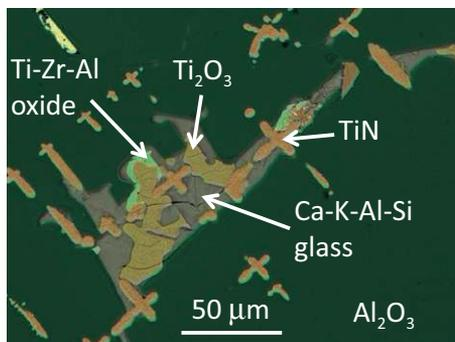
**Figure 4.** Energy-dispersive X-ray spectroscopy–scanning electron microscopy composite element map of type N and type S melts from Mount Carmel, Israel. TiN appears to reside in cavities in skeletal crystal; type S pocket shows both straight and locally lobate boundaries, characteristic of skeletal growth. Dark needles in glass are anorthite.
