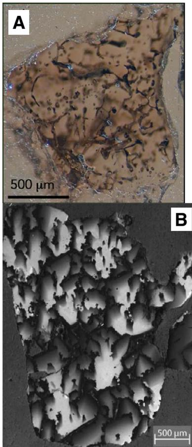
**Figure 1. Non-gem corundum from Mount Carmel, Israel. A: Crystal aggregate with three-dimensional network of melt inclusions (dark blebs, curvilinear strings). B: Cathodoluminescence image of aggregate of zoned crystals; darker areas are higher in Ti and typically adjoin melt pockets.**
