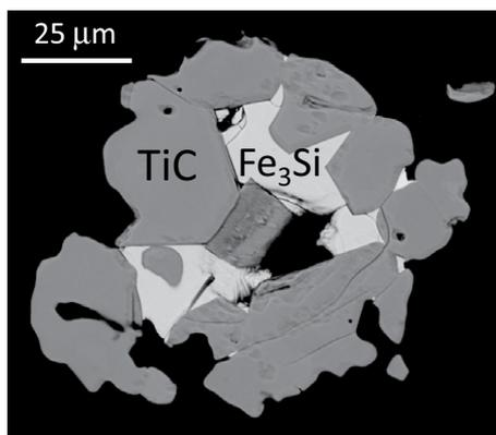
**Figure 3.** Backscattered electron (BSE) image of type A melt inclusion in corundum from Mount Carmel, Israel; crystals of TiC surround a pool of  $\text{Fe}_3\text{Si}$ .
